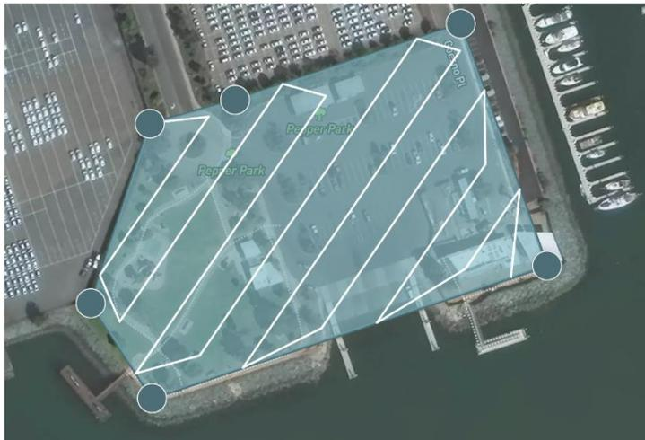
1. **Maintain proper and constant overlap** - It is recommended to maintain at least 75% overlap along the flight path and 60% overlap in the orthogonal direction. (80% front overlap and 65% side overlap is recommended).
