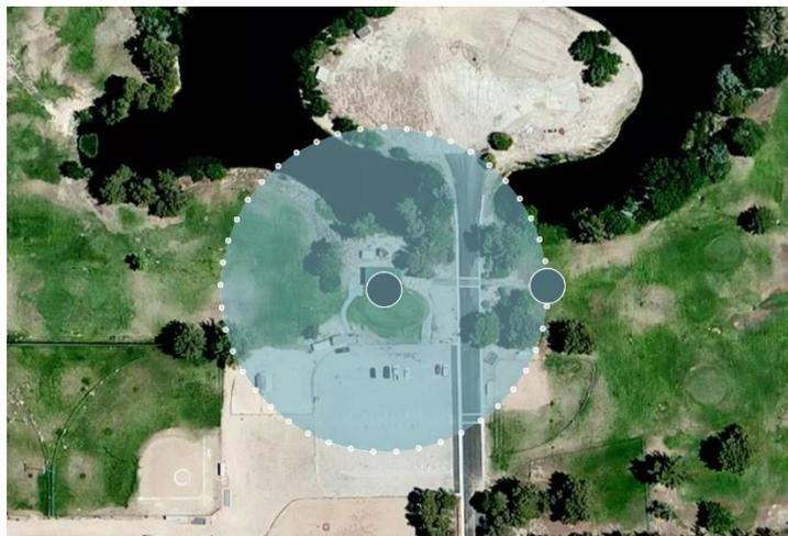
1. **Maintain proper overlap** - It is recommended take enough images at a constant distance on the circle between them to maintain a good overlap. For example, for a 40 meter radius circle at a height of 40 meters, take about 45 images.
